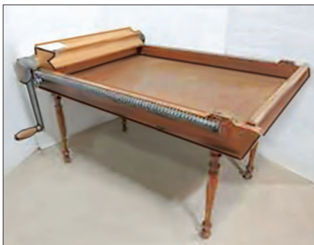
Fig. 10.23 : Wooden Butter worker
