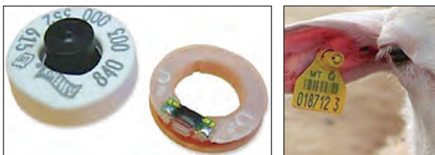
Fig. 1.8 : Parts of RFID ear tag
