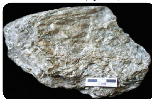
Fig. 2.24 : Muscovite exhibiting Schistose structure
