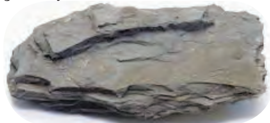
Fig. 2.22 : Slate exhibiting slaty cleavage
