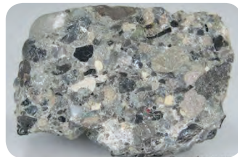
Fig 2.16 : Conglomerate showing clastic texture
