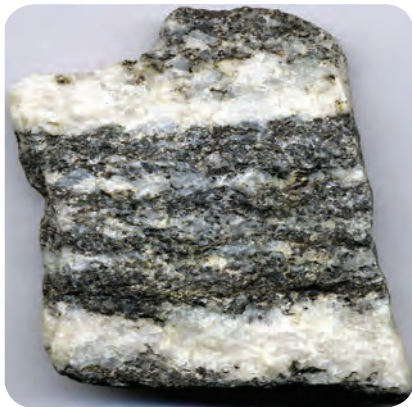
Fig. 2.25 : Gneissose structure Alternate bands of Biotic and Quartz exhibiting Gneissose structure
