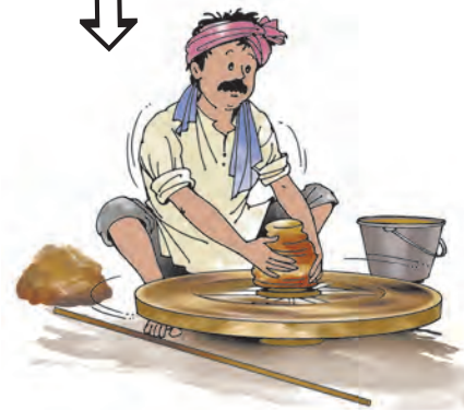
He turns the kneaded clay on a wheel to shape the pot.
