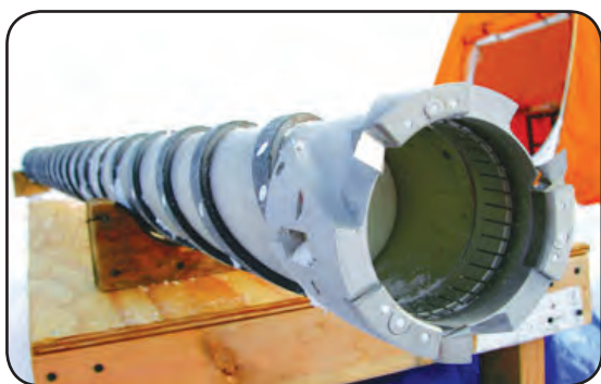
Fig. 5.8 Ice driller used for taking sample from ice
